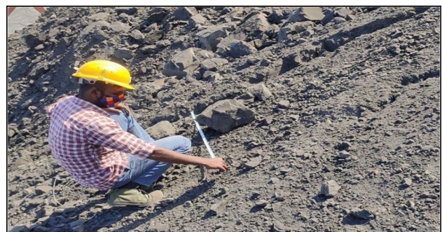
Fig. 7 Estimating distance of back break created during blasting
